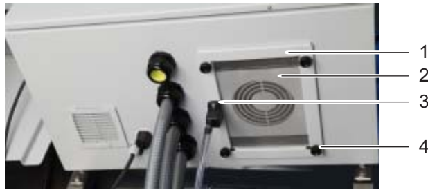
figure 4-18 Mounted bug screen and condensate drain adapter
