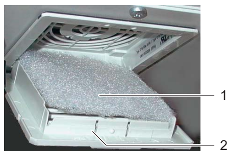
figure 6-16 Exchanging the lower filter mat
