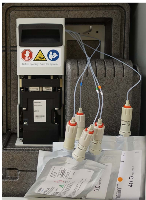
figure 6-6 ChemBags removed to be exchanged
