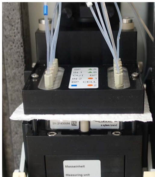
figure 6-2 Removing the liquids remains with absorbent, lint free paper
