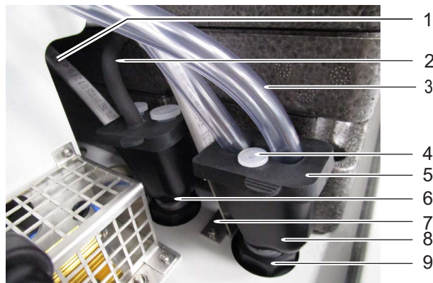
figure 4-26 Collection funnel for the separate discharge of all liquids
