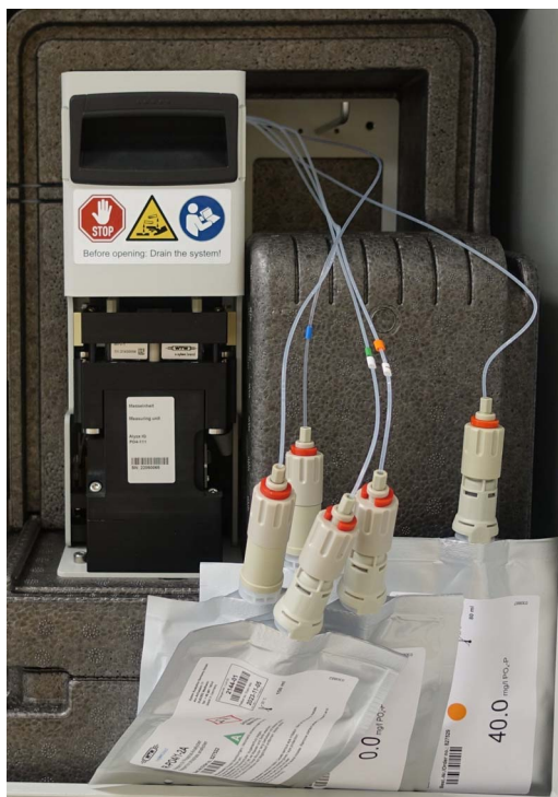
figure 6-19 ChemBags removed from the supporting rod
