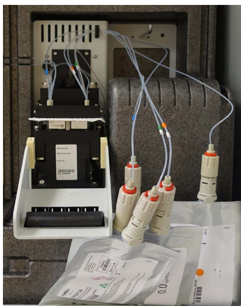
figure 6-20 Absorbent paper in the receptacle of the MultiPort valve
